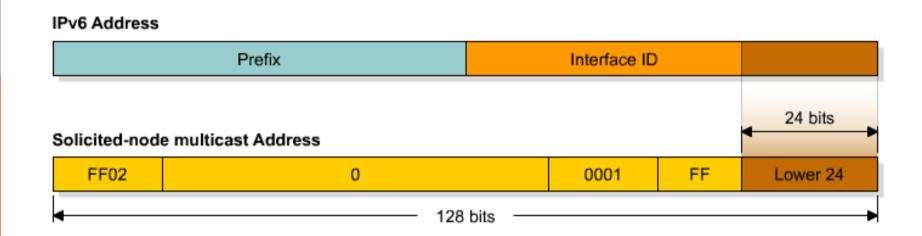
Solicited-node multicast address consists of FF02:0:0:0:0:1:FF::/104 prefix joined with the lower 24 bits from the unicast or anycast IPv6 address
