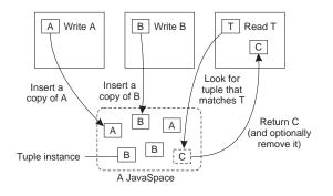
Write: A copy of a tuple (tuple instance) is stored in a JavaSpace
